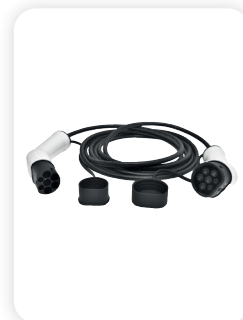
Cavo ricarica 5m modo 3 da 32A spina/connettore 3P+N+PE IP54 Charging cable 5m mode 3 of 32A plug/connector 3P+N+PE IP54 COD. ECCAB5M
